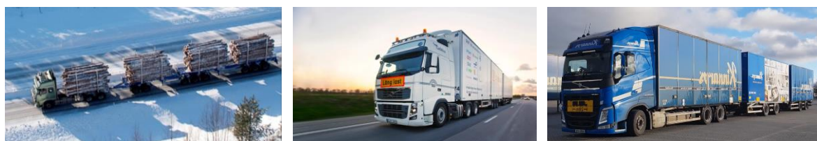
Figure 3 – Examples of tested LVCs in Sweden From left to right: ETT vehicle, DUO-trailer, DUO-CAT
