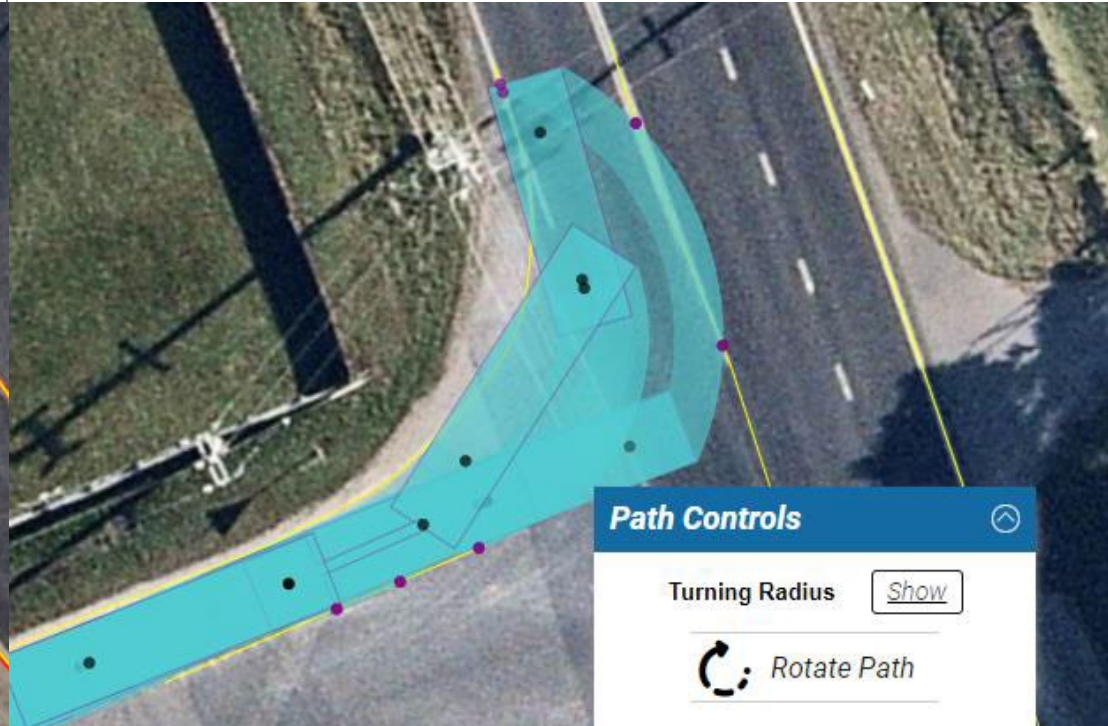
Collision points (purple) visualise the degree of obstruction encroachment
