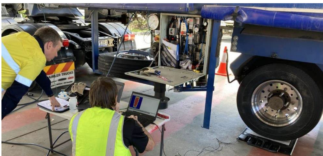
Figure 6 Recording tyre contact pressure distribution
