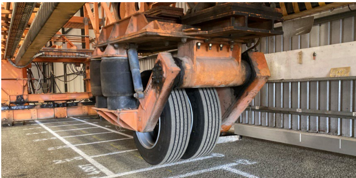
Figure 8 Trafficking of the test pavement
