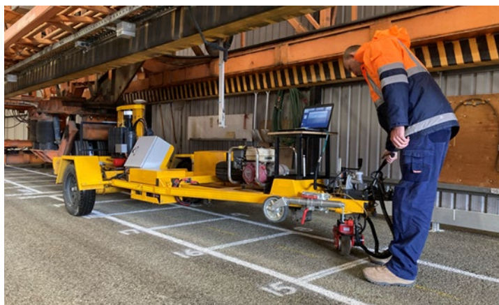
Figure 5 Deflection testing at ALF site using the FWD
