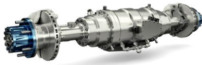
Figure 5 - eTransport- axle (BPW, 2017)
