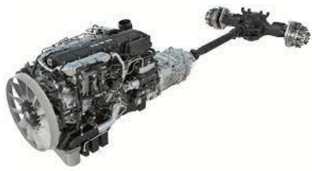
Figure 1 – ICE- powertrain (MAN, 2020) Figure 2 – ICE- powertrain (Mercedes-Benz)
