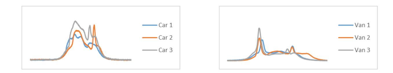
Typical measured chassis responses of a passenger car and van
