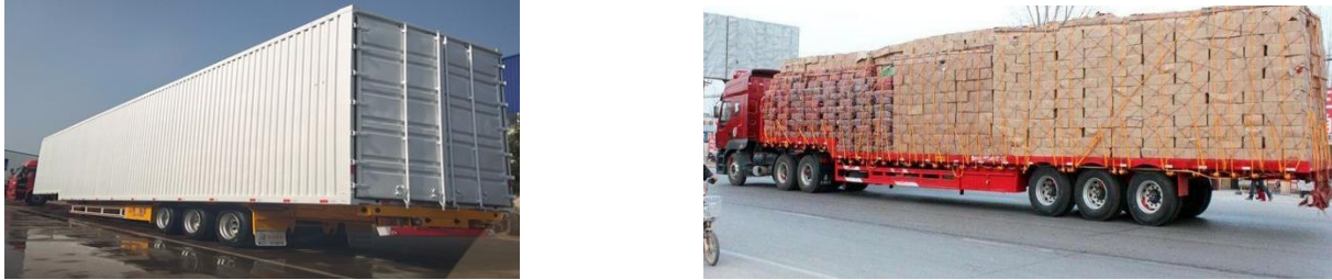
Figure 1 – Left: Oversized container box on a compliant semitrailer chassis Right: Gooseneck flat low bed semitrailer
