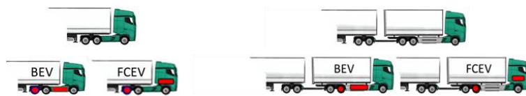
Figure 2 – Modular Heavy Duty (HD) Battery Electric Vehicles (BEVs) and Fuel Cell Electric Vehicles (FCEVs).
